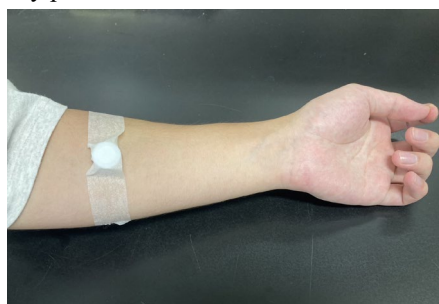
Figure 1 Sampling of human skin gases using the PFS at a forearm of volunteer.
