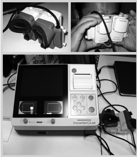
図1 電子瞳孔計 (Irisrecorder Dual) Fig. 1 Videopupulography (Irisrecorder Dual)
