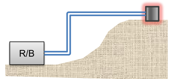
Location of power generator for disaster preparedness
