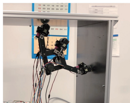
Fig.1 Mobile robot for steel bridge maintenance
