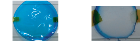
Without treatment OH* (high humidity) ヒドロキシラジカル検知用インジケータ Thin film indicator that specifically reacts to OH*
