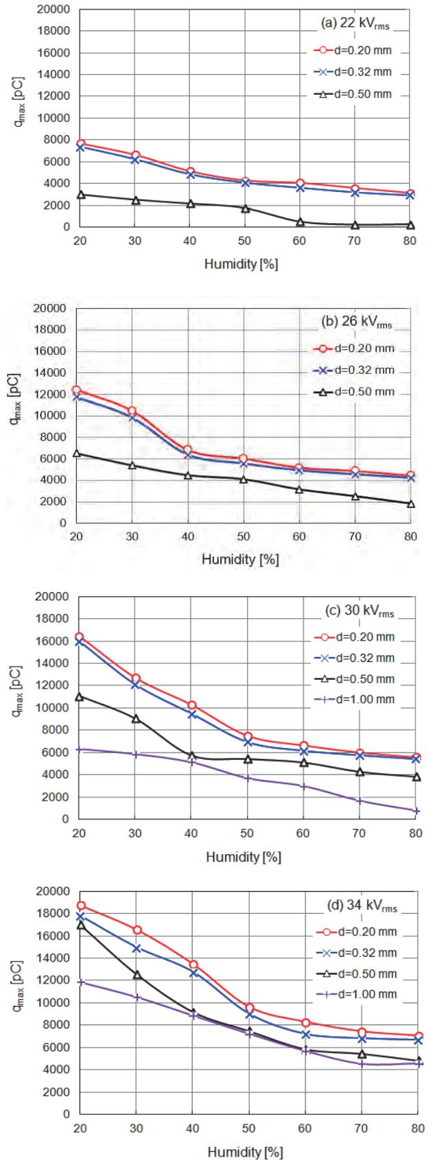
Fig.7 Maximum magnitude  $q_{max}$  of negative corona discharge pulses as a function of humidity for applied voltage: (a) 22, (b) 26, (c) 30, and (d) 34 kV<sub>rms</sub>.
