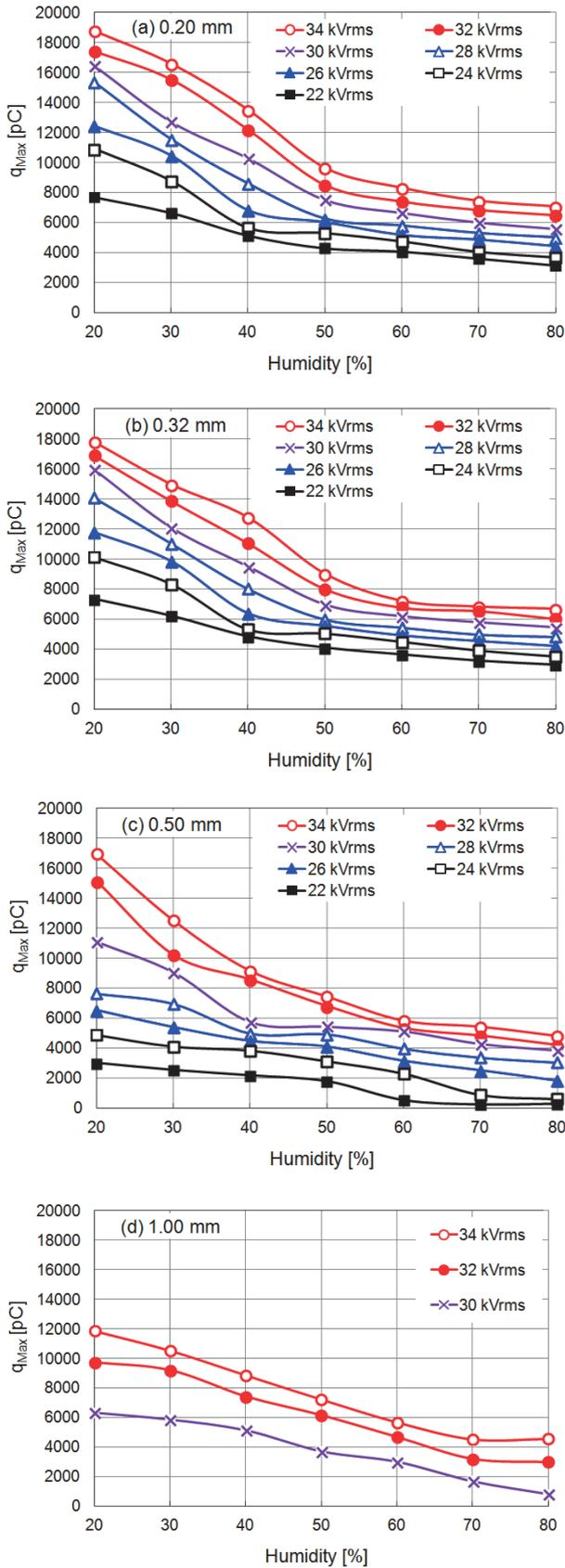
Fig.4 Maximum magnitude  $q_{max}$  of negative corona discharge as a function of humidity for wire electrode diameters: (a) 0.20, (b) 0.32, (c) 0.50, and (d) 1.00 mm.
