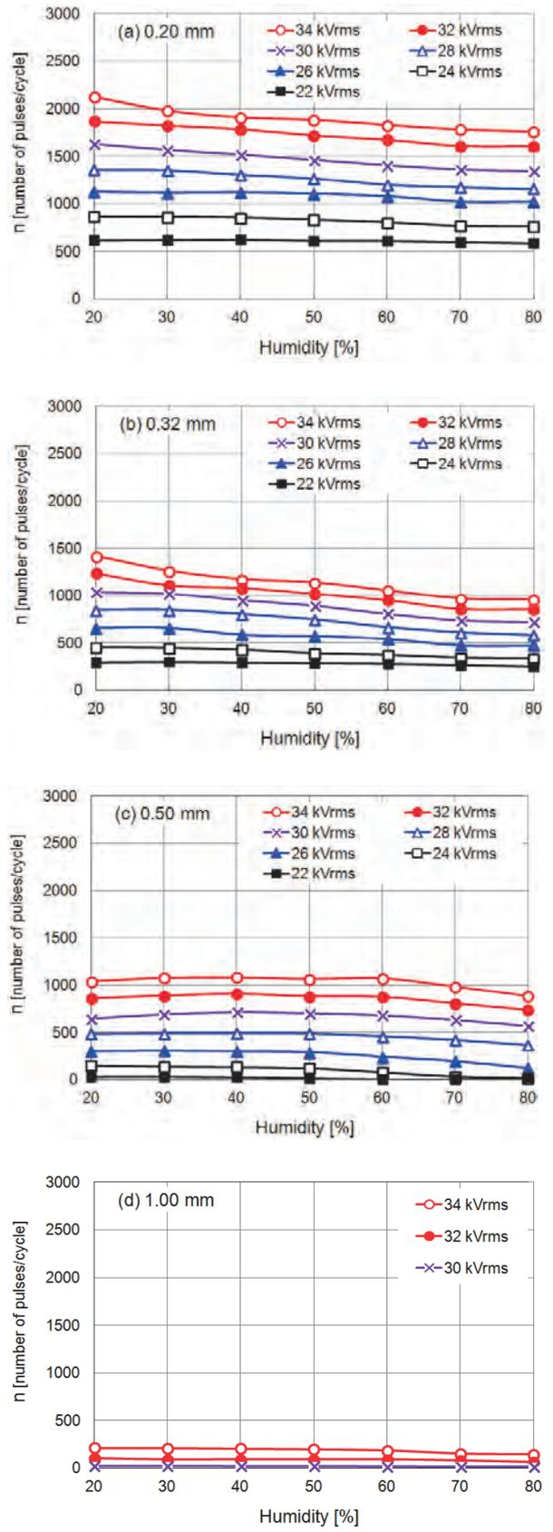
Fig.5 Number of pulses per cycle  $n$  of negative corona discharge as a function of humidity for the wire electrode diameters: (a) 0.20, (b) 0.32, (c) 0.50, and (d) 1.00 mm.
