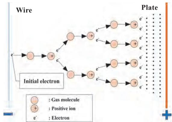
Fig.9 Ionization process by electron collision with neutral gas molecules.
