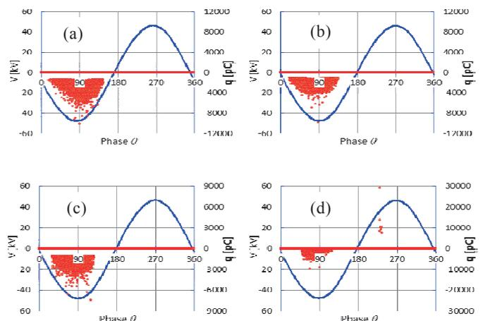
Fig.2 AC corona discharge pulses with gap length of 30 mm, applied voltage  $V$  of 34 kV<sub>rms</sub>, and wire electrode diameters: (a)  $d=0.20$ , (b)  $d=0.32$ , (c)  $d=0.50$ , and (d)  $d=1.00$  mm.
