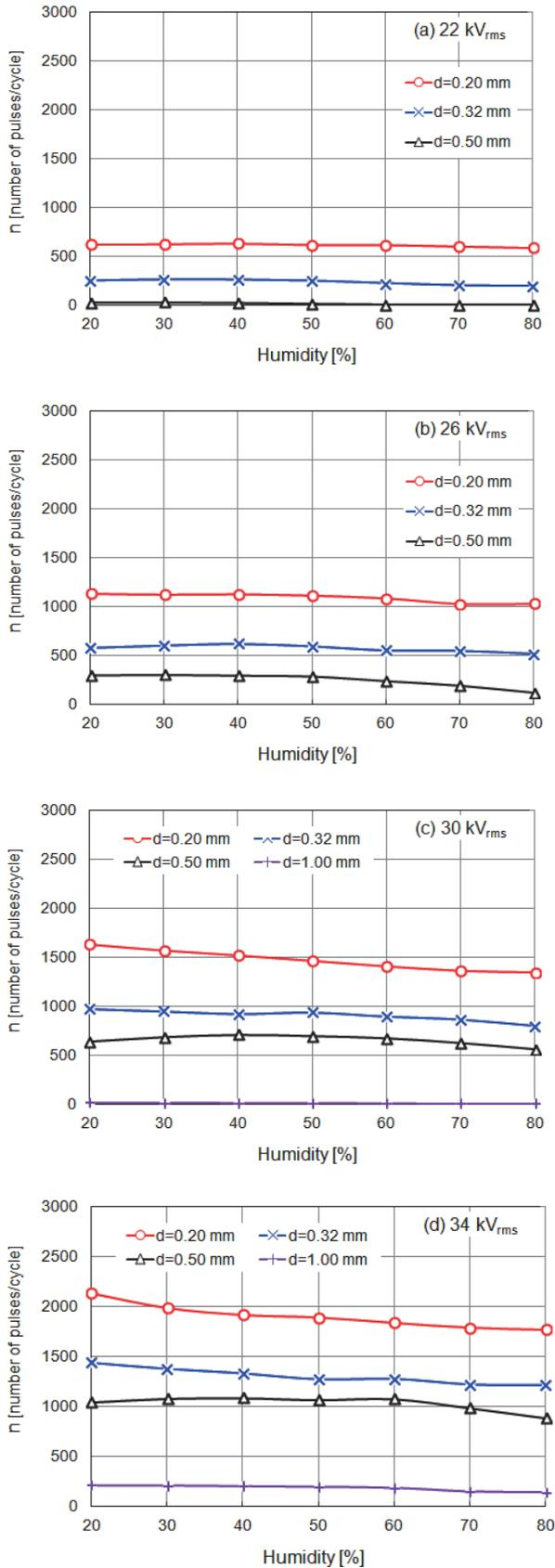
Fig.8 Number of pulses per cycle  $n$  of negative corona discharge pulses as a function of humidity for applied voltage: (a) 22, (b) 26, (c) 30, and (d) 34 kV<sub>rms</sub>.
