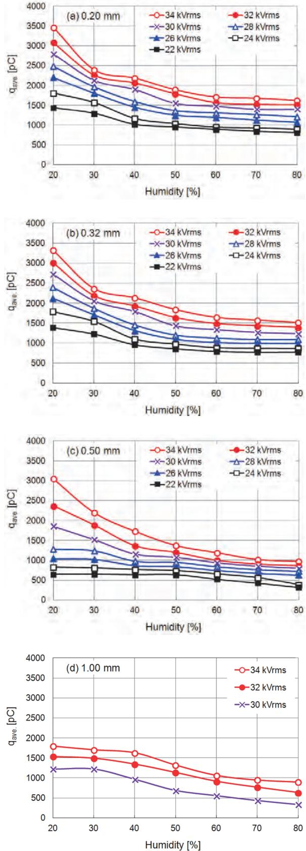
Fig.3 Average magnitude  $q_{ave.}$  of negative corona discharge as a function of humidity for wire electrode diameters: (a) 0.20, (b) 0.32, (c) 0.50, and (d) 1.00 mm.
