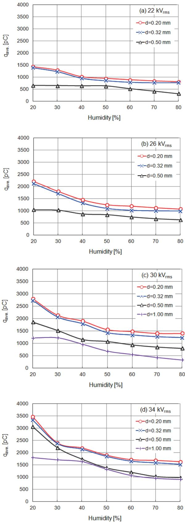
Fig.6 Average magnitude  $q_{ave.}$  of negative corona discharge pulses as a function of humidity for applied voltage: (a) 22, (b) 26, (c) 30, and (d) 34 kV<sub>rms</sub>.
