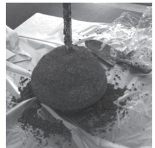
Fig.10 Shape of the solidified soil mass.
