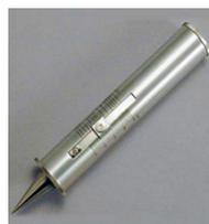
Fig. 2 Yamanaka type soil hardness meter.
