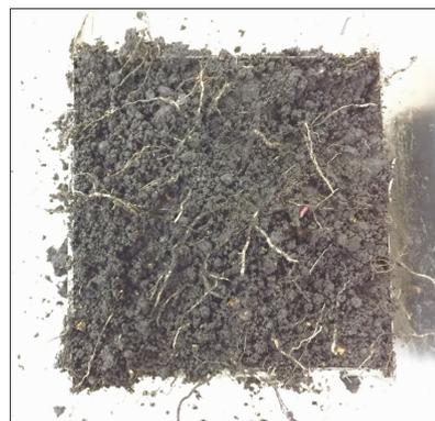
Fig. 24 Roots of cross section in shear frame after shearing.
