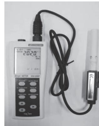
Fig.6 Portable electrical conductivity meter.
