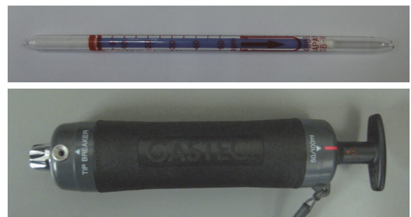
Fig. 2 O 3 detection tube and gas sampler.
