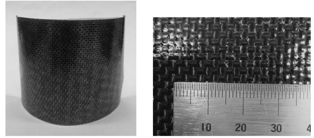
Fig. 2 Rectangular CFRP prepreg cut out for lamination.
