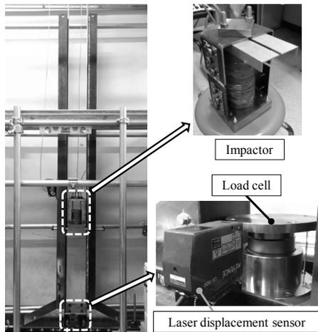
Fig. 5 Constructed drop weight tester.
