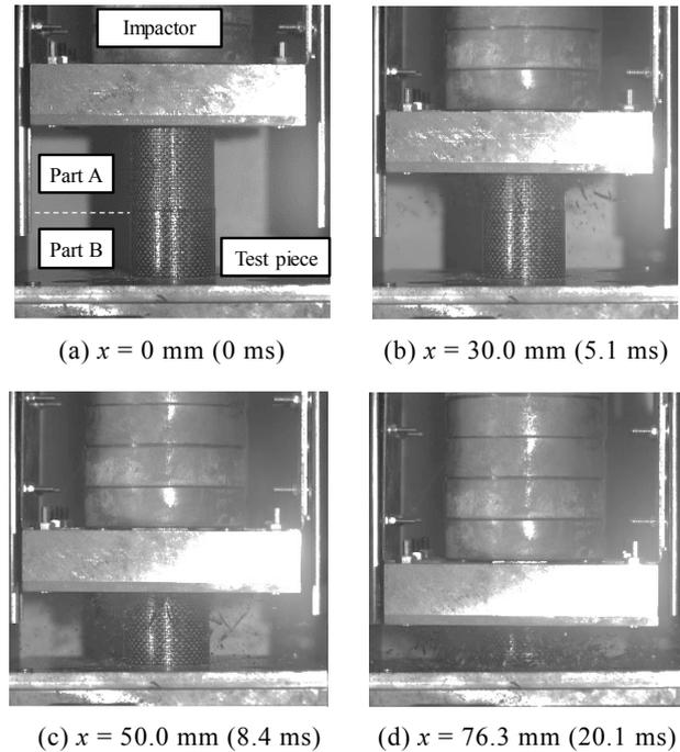
Fig. 11 Crushing of CFRP test piece.
