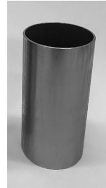
Fig. 3 Metal jig for CFRP lamination.
