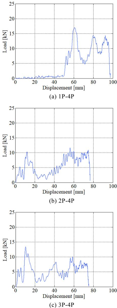
Fig. 12 Load–displacement diagrams of CFRP test pieces.
