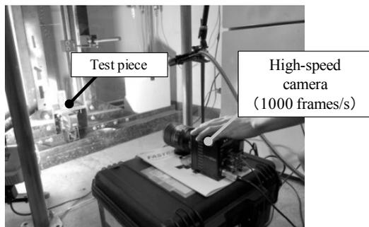
Fig. 10 High-speed camera
