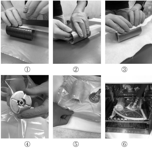
Fig. 4 Procedures for lamination and curing.
