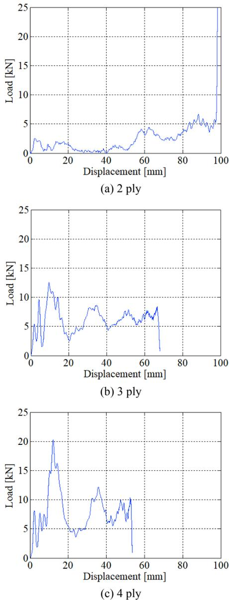
Fig. 7 Load–displacement diagrams of CFRP test piece.
