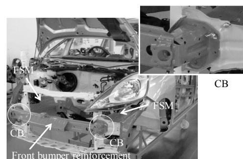
Fig. 1 Structure of front of vehicle, consisting of FSM and CB.
