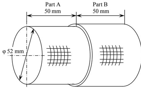
Fig. 9 Schematic of CFRP test piece with different ply numbers.
