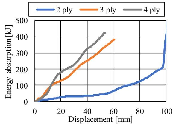
Fig. 8 Relationship between energy absorption and displacement.
