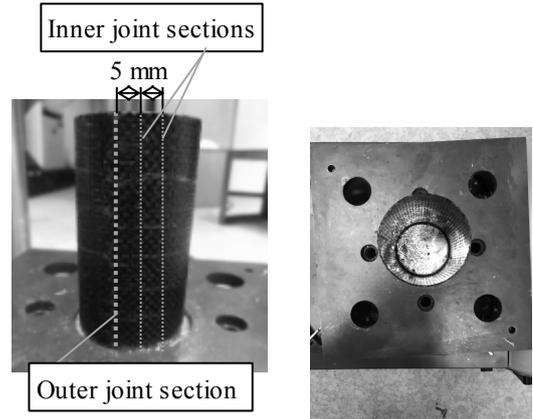
Fig. 6 Test piece fixed with fusible alloy.
