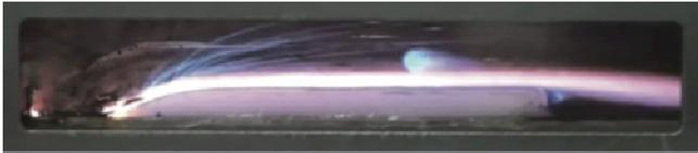
Fig.1 Combustion image of wax fuel<sup>1)</sup>
