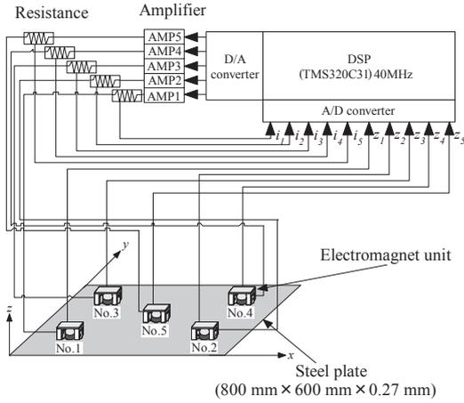
Fig. 1 Electromagnet control system
