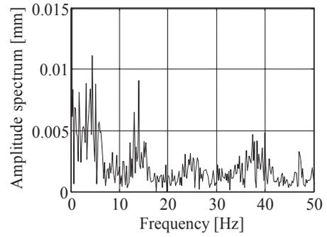
Fig. 7 Vibration of a levitation steel plate for 1-DOF model ( $\theta = 0^\circ$ )
