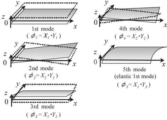
Fig. 3 Mode shapes of the levitated steel plate
