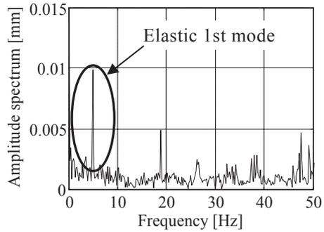
Fig. 8 Vibration of a levitation steel plate for 1-DOF model ( $\theta = 7^\circ$ )
