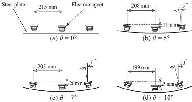
Fig. 4 Relationship between tilt angle of electromagnets and shape of steel plate
