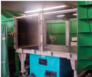
Fig.2 Ground board and test section
