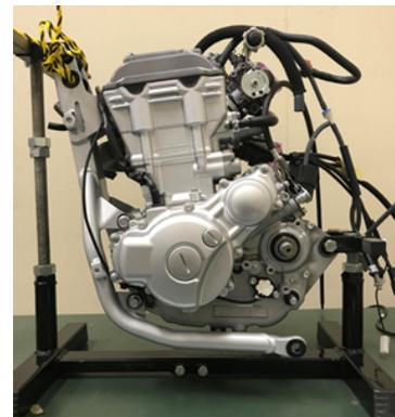
Fig. 3 Internal combustion engine YAMAHA G363E.
