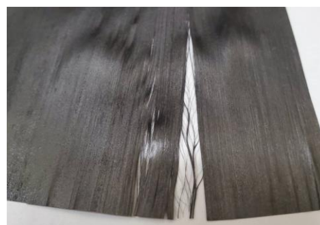
(b) Unidirectional carbon fiber in UD prepreg
