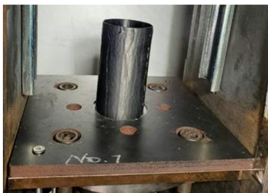
Fig. 7 Photograph of specimen fixation method.
