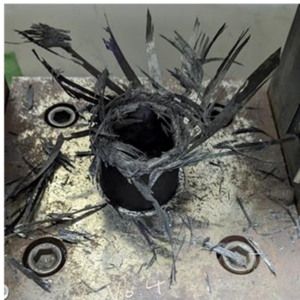
(a) Specimen C [45^\circ/0^\circ/-45^\circ/0^\circ/45^\circ]
