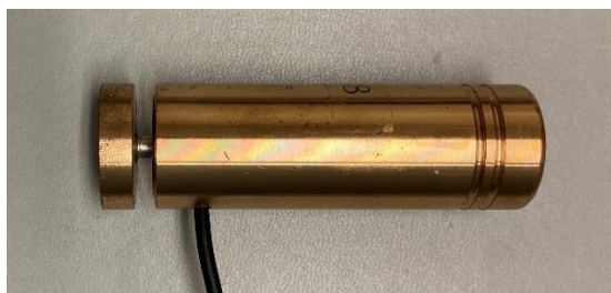
Fig. 1 Giant magnetostrictive actuator.
