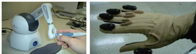
Fig.8 PHANToM Omni™ (left) and Cyber Touch™ (right).
