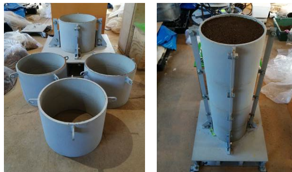
Figure 1. Steel mold (left) and test specimen (right)
